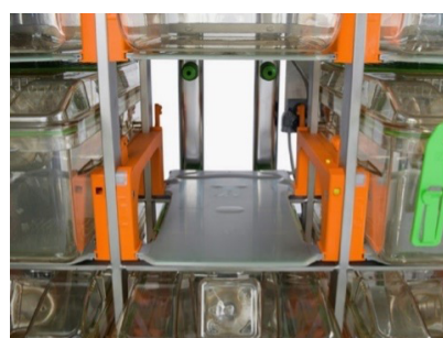
Picture 2. On the left is represented a picture of a mouse cage slot in the Tecniplast DVC® Rack for home-cage monitoring. The gray board contains 12 electrodes arranged in a grid as represented in the diagram. When a cage is inserted in a slot, the board is positioned right under the floor of the cage. A miniature electromagnetic field is generated between each electrode. Electrodes record individually the intensity of the electromagnetic fields at 4 Hz. When the mouse is above an electrode, the intensity of the electromagnetic field is modified thus enabling the localization of the mouse in its cage with a high temporal resolution.
